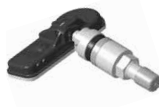
Moment mutter 8.0 Nm Moment ventilnål 0.4 Nm
